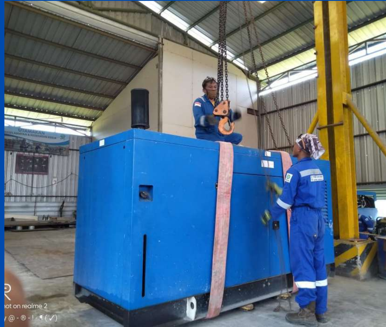
PERTAMINA HULU ENERGI WEST MADURA OFFSHORE Overhaul Compressor and Replacement of Skid and enclosure
